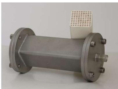
Fig. 3 - Binderfree zeolite 13X monolith.
