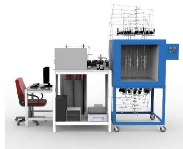
Fig. 1. Experimental set-up of the gas phase simulated moving bed.
