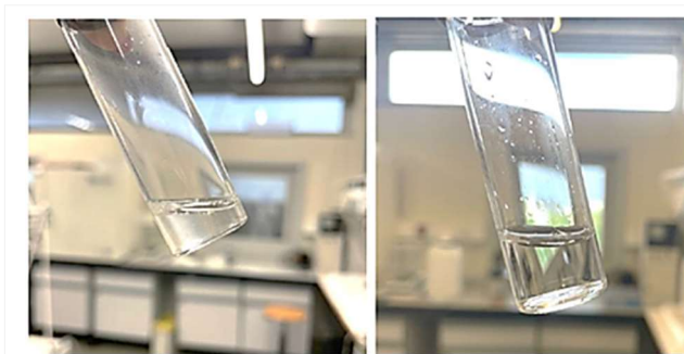
Fig 1. Example of application of the cloud-point method: turbid mixture – left; clear mixture – right.
