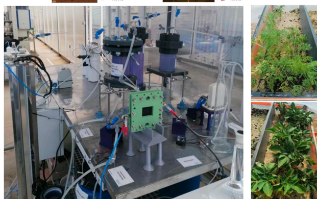
Fig 2. Scheme of the multi-barrier approach to treat the municipal WWTP effluent, and photographs of the prototype treatment plant and the agricultural tests.
