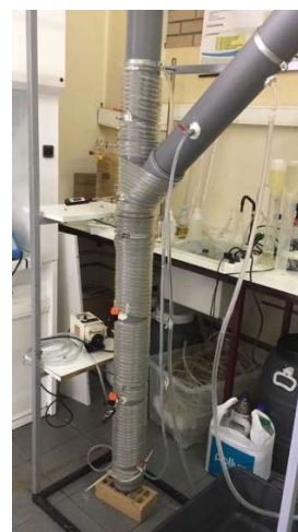
Fig 2. Experimental setup – upflow anaerobic sludge blanket digester reactor (UASB).
