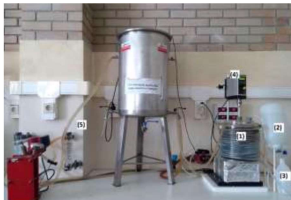
Fig 1. Biogas production system at mesoscale.
