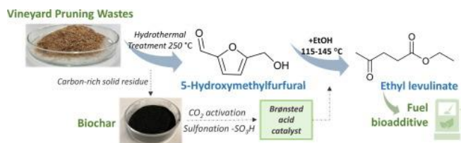
Fig 2. Schematic illustration of the conversion of HMF to EL over biochar catalysts produced from vineyard pruning wastes.
