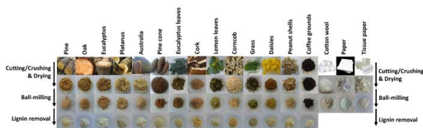
Fig 4. Photographs of the waste materials before and after cutting/crushing, drying, ball-milling, and lignin removal.
