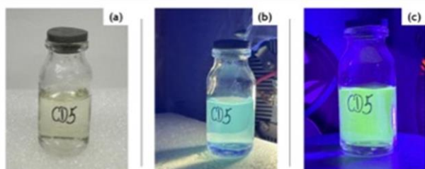
Fig. 1. Images of an aqueous suspension prepared with CD 5 when subjected to (a) natural light, and (b) 365 nm and (c) 401 nm LED quantum yields up to 25.4%. Moreover, exposing the CDs to different
