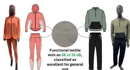
Fig 2. Prototype clothes with pockets created using functional textiles with EMI shielding properties for low-frequency radiation attenuation.
